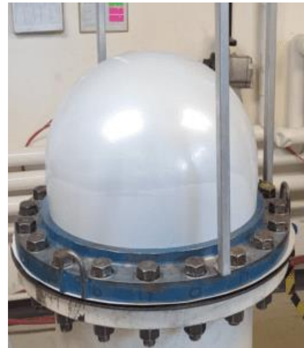
Multiaxial testing of 50 mil LLDPE, Layfield 1 mil = 0,0254 mm
