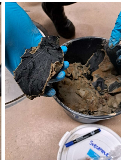
Excavated soil in Heikkilänkangas-Oulu. unoxidized clay (left-Photograph-Veikko Pekkala) and oxidized clay (middle and right-Photograph Heli Kivisaari)
