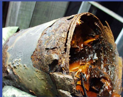
Severe corrosion and deterioration of bitumen painted steel cap after 30 years in service
