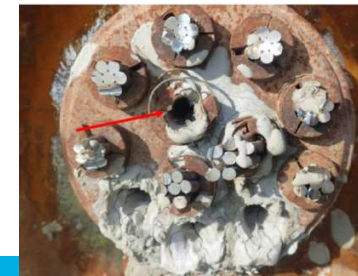
Removal of protective cap reveals severely corroded barrel and wedges after 11 years in service
