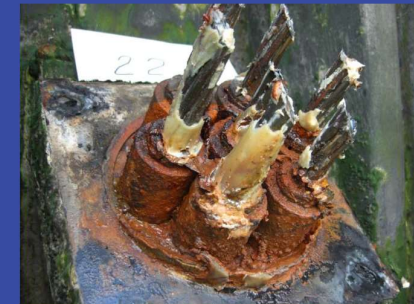
Removal of protective cap reveals severely corroded barrel and wedges after 11 years in service
